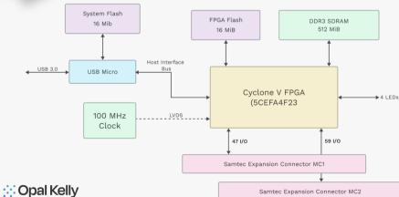
Host Interface USB 3.0 Type C, SuperSpeed FrontPanel Support **FPGA** 5CEFA4F23C7N 512 MiByte DDR3, 32-bit wide data interface Memory **NV Memory** 16 MiB System Flash 16 MiB FPGA Flash Oscillator 100 MHZ FPGA I/O Voltage Up to +3.3V
